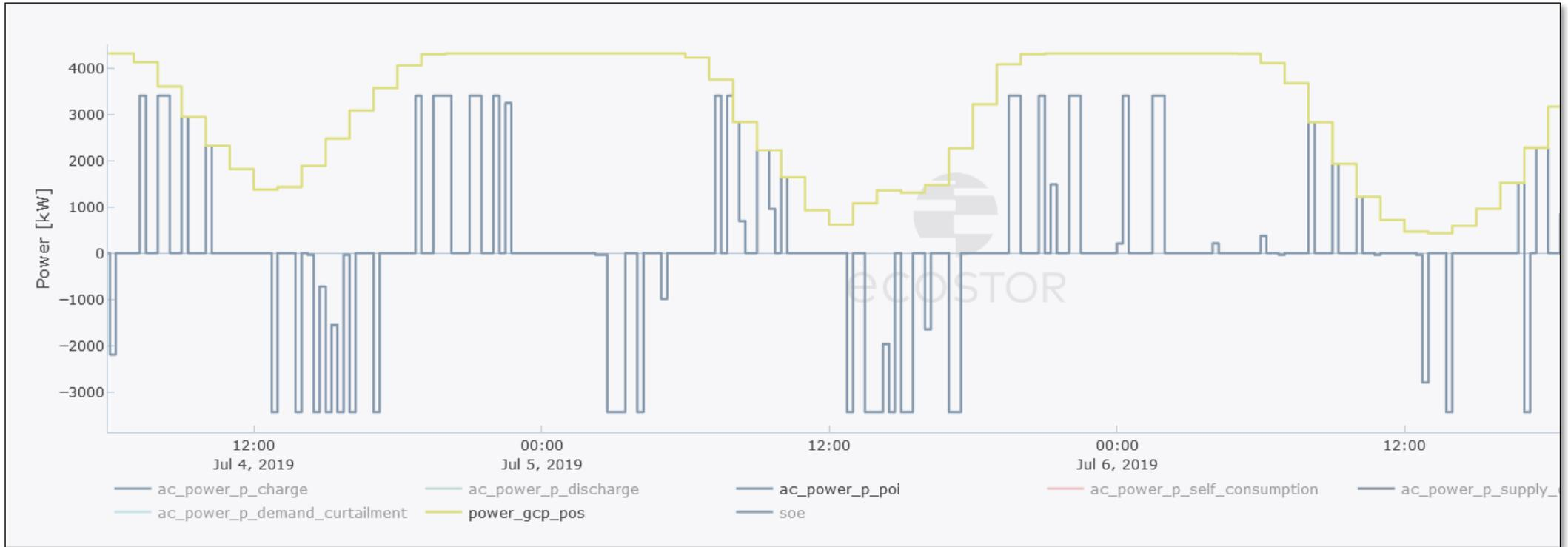
Colocation PV & storage - storage power profile (ID) vs. available power at grid access point
